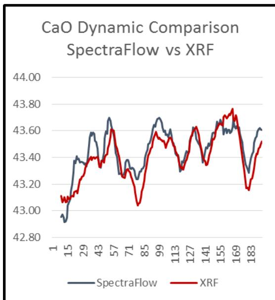
Fig 4: Comparison of CaO measured by SpectraFlow and XRF over 190 samples (8 days)
