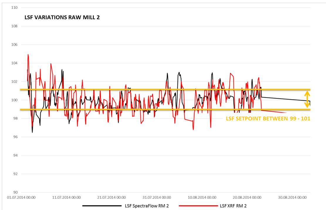
*Fig 10: LSF Variations at Raw Mill 2 measured by SpectraFlow and XRF. The LSF Standard Deviation based on XRF is 2.80, while based on SpectraFlow 1.45. The setpoint was frequently changed by the operators between 99 and 101 and therefore the corrected values are at approx. 1.8 (XRF based) and well below 1 (SpectraFlow based)*
