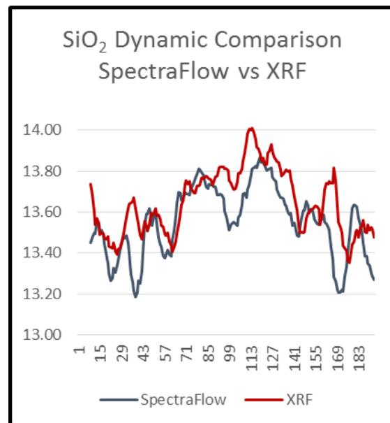
Fig 5: Comparison of SiO<sub>2</sub> measured by SpectraFlow and XRF over 190 samples (8 days)
