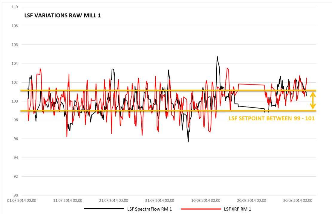
*Fig 9: LSF Variations at Raw Mill 1 measured by SpectraFlow and XRF. The LSF Standard Deviation based on XRF is 2.69, while based on SpectraFlow 1.65. The setpoint was frequently changed by the operators between 99 and 101 (=Standard Deviation approx. 1), which means the LSF Standard Deviation includes these setpoint changes. To see the real LSF Standard Deviation without any setpoint changes these values have to be corrected by 1.*
