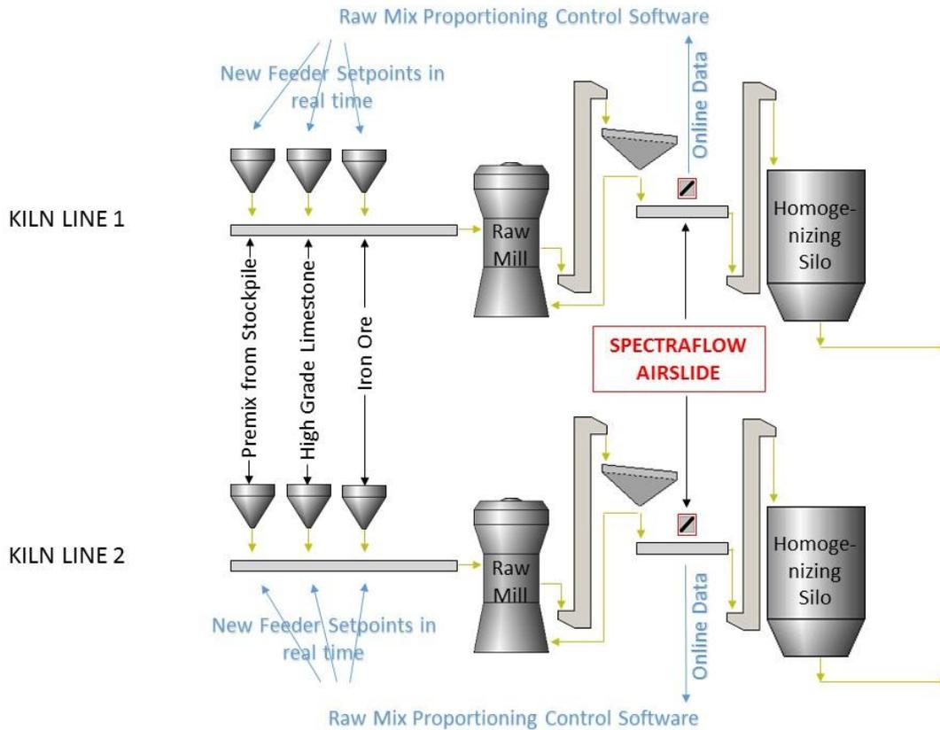
Fig 8: Flow sheet of the Raw Mill operation at Kipaş Cement. Beside the Premix from the stockpile also High Grade Limestone and Iron Ore is used to achieve the LSF setpoint at the raw mill. The SpectraFlow Online Analyzers are installed after the raw mill and the control software is adjusting the weight feeders before the raw mill
