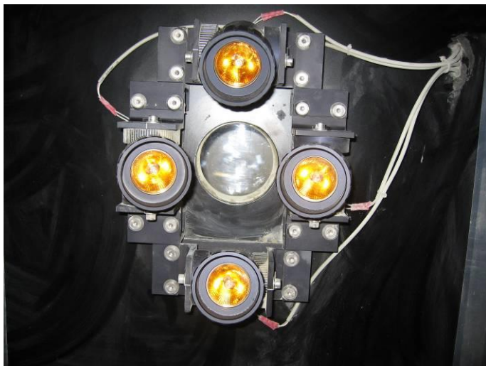
Inside view of illumination head showing lights and spectrometer entry
